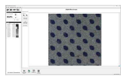
discover any soiling or exposure errors now that the structure of the raster dots is visible.
